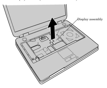
Figure 4-17 Removing the display assembly (3)
